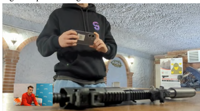
Figure 23. Field testing of the CEASEFIRE mobile weapons-recognition application at a shooting range in Poznań, Poland
